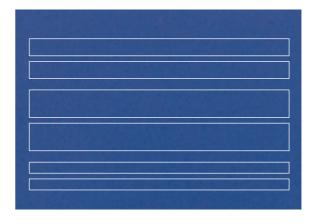
When cutting dark-colored material using Direct Cut, using a white or other light-colored pen to draw the cutting lines on the back of the material helps ensure better recognition.
